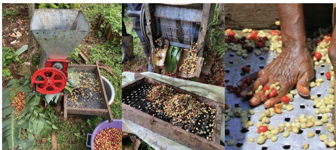
Figure 8. To the left: An outlived pulping machine separates most of the beans from the berry skin (pulp).
